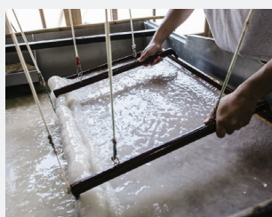
6. Mixing the mucilage and tree fibers.
